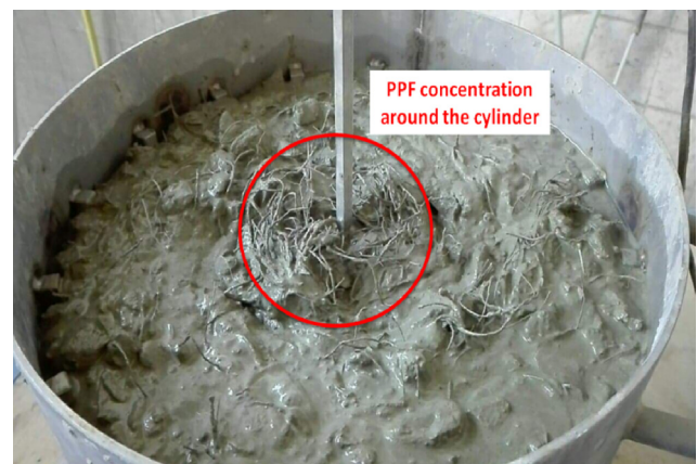
Fig. 13. The 54 mm PPF concentration around the vane during the test.
